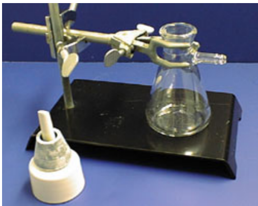
clamp a side arm flask securely to a ring stand
