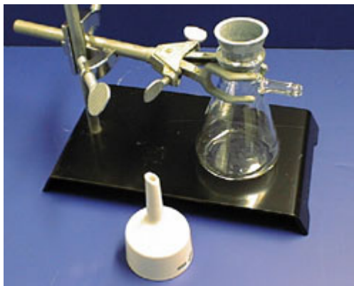
place the rubber adaptor in the side arm flask
