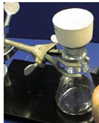
connect the side arm vacuum source - always walled tubing , since Ty will collapse under redu
